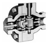
The straight-through flow path of a sliding gate valve reduces velocity and turbulence and leads to quiet operation and reduced wear.
