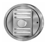
Sliding gate seats are made up of a disc and plate, both slotted with openings that align to allow the required flow to pass through the orifices.
