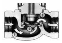
In conventional rising stem globe style valves, the flow changes directions three times as it follows an "S" path. This leads to greater velocity, turbulence, noise and more wear on the seating components.
